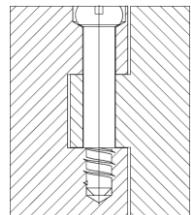
**DJ-Screws with ISS Technology for combination frames**
